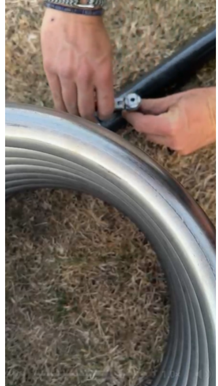
Slide on the hose clamp first.
