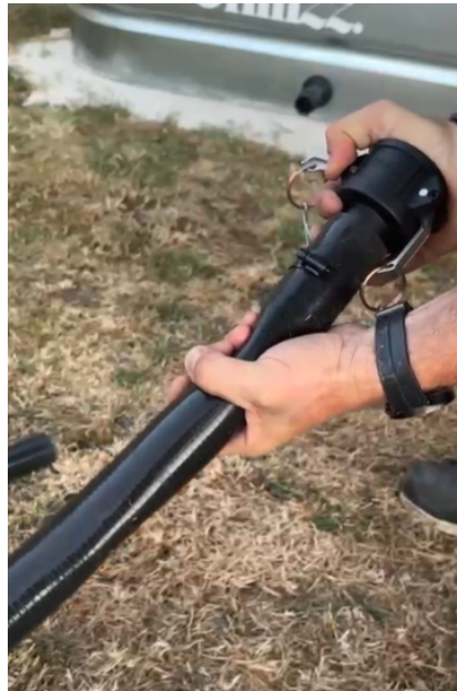
Position the clamp behind the barb.
