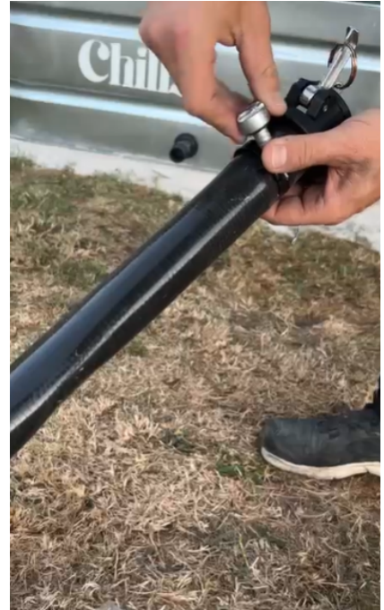
Prepare the camlock connection.
